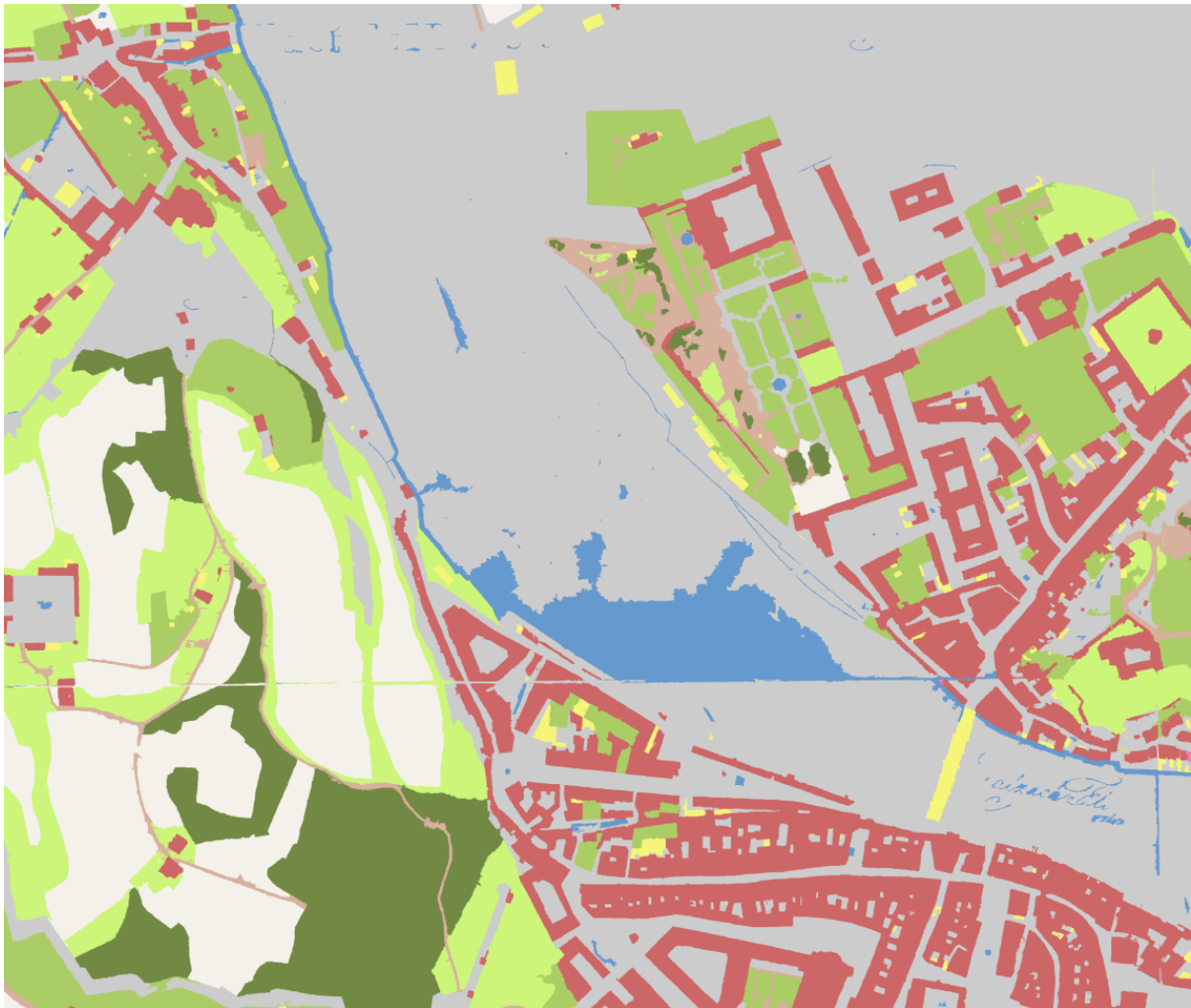
Figure 17: Misclassifications at the Salzach river. Some outlines around letters remain, as they were falsely classified as water and subsequently missed in the reclassification phase, which aimed at removing letters, lines, and no data areas from the classification. A horizontal line is also visible, which was likely caused by the mosaicking of the map sheets after the scanning of the original map source.
