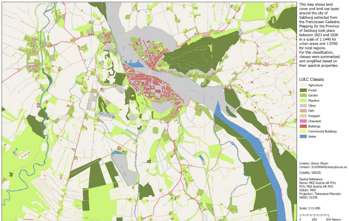
Figure 12: Final LULC classification for the Salzburg area. The area consists of two map images ('Salzburg-West' and 'Salzburg-East') that were processed and validated separately and then merged in GIS. The 'Salzburg-East' area was used for the training of the classification model, while the 'Salzburg-West' area was used in the development of the classification workflow and the final accuracy assessment.
