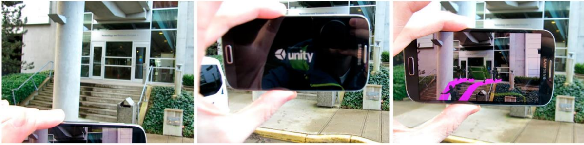
Figure 3: Result of the AR emergency simulation. Simulated agents are superimposed onto the screen of the device when the camera recognizes the surrounding (Lochhead & Hedley, 2019, p. 200).
